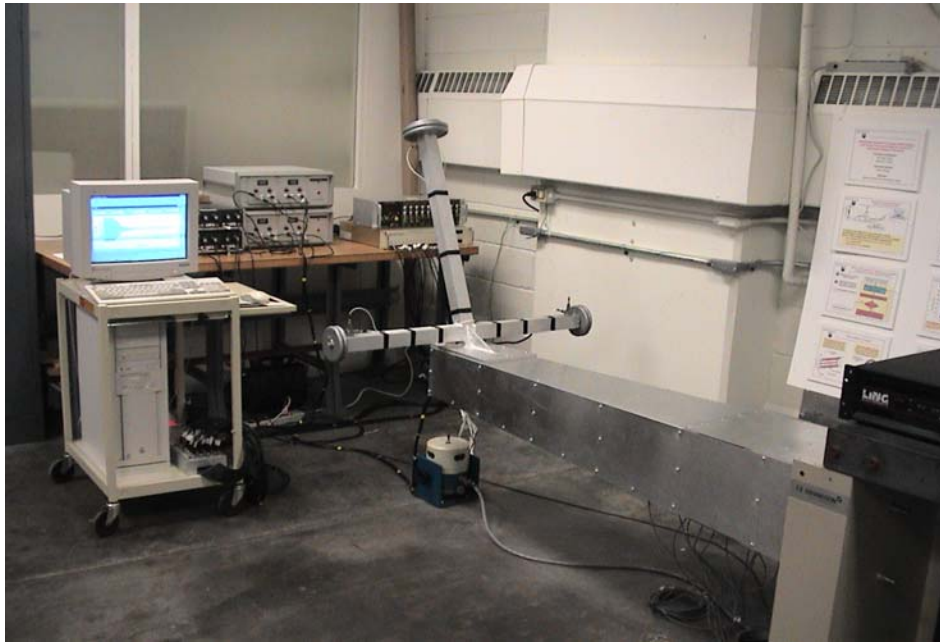
Figure 5. Scaled helicopter tailboom structure with built-in piezoelectric actuators
