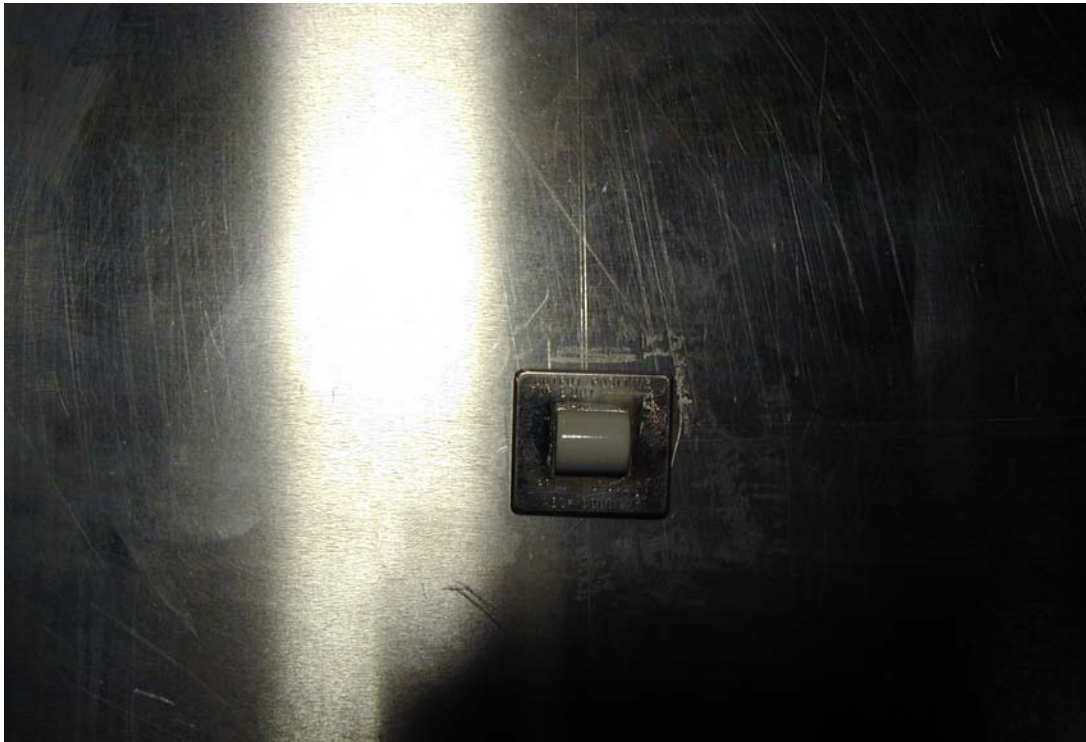
Figure A-8. The ground plane B-dot sensor
