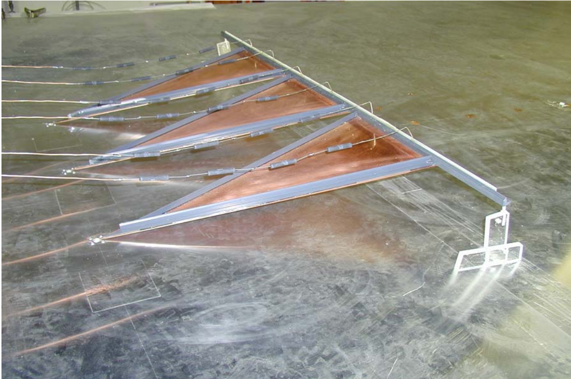
Figure A-5 The geometry associated with three TEM horn array (side view).
