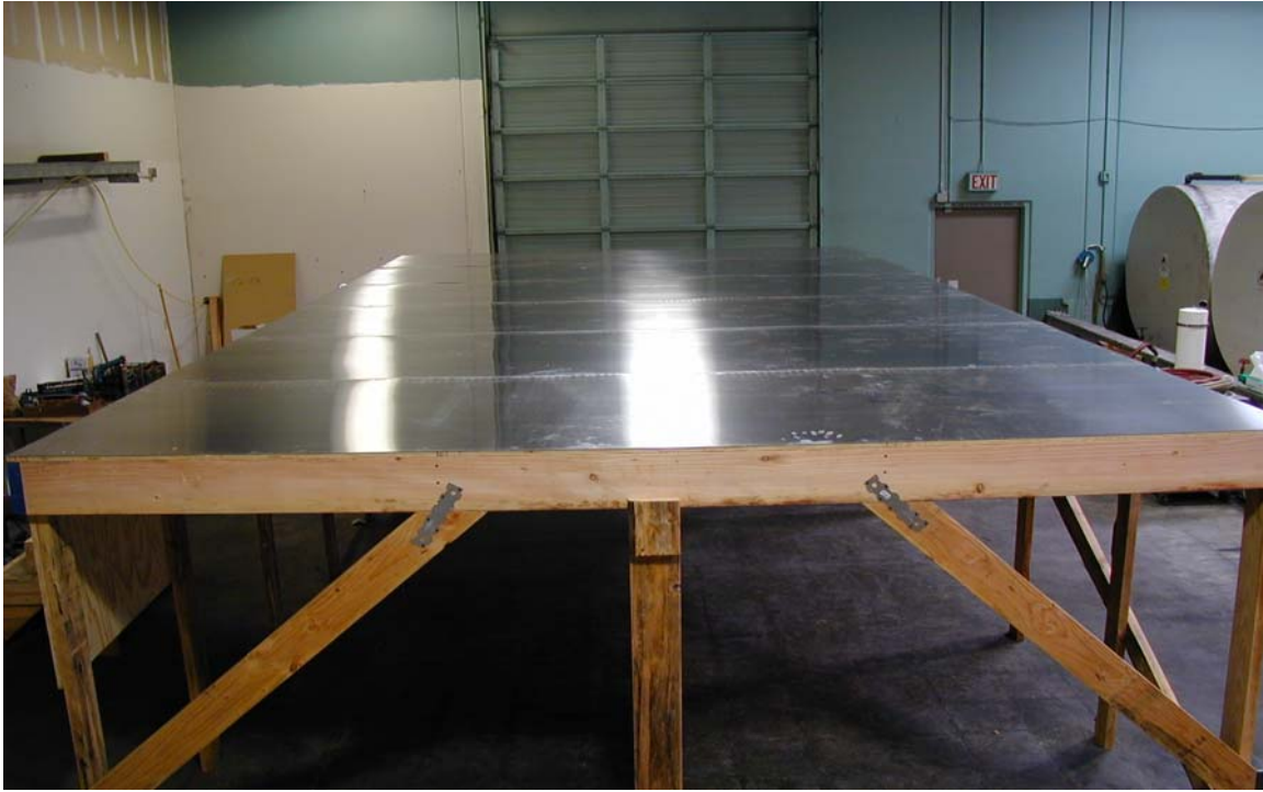
Figure A-1. Experimental table used as a ground or image plane
