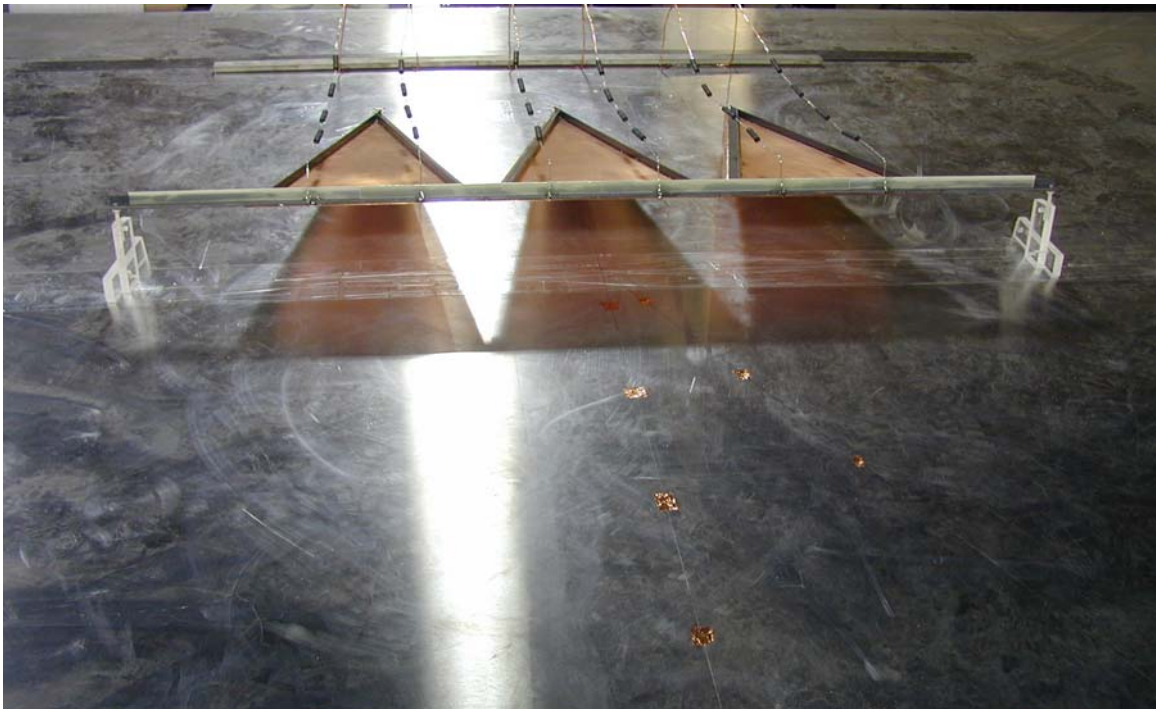
Figure A-6. The geometry associated with three TEM horn array with high-inductance load (front view).
