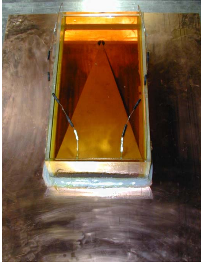
Figure D-1. View of a single TEM horn in an oil bath; energized by a hv ( \sim 300 kV) fast rising ( \sim 100 ps) pulse
