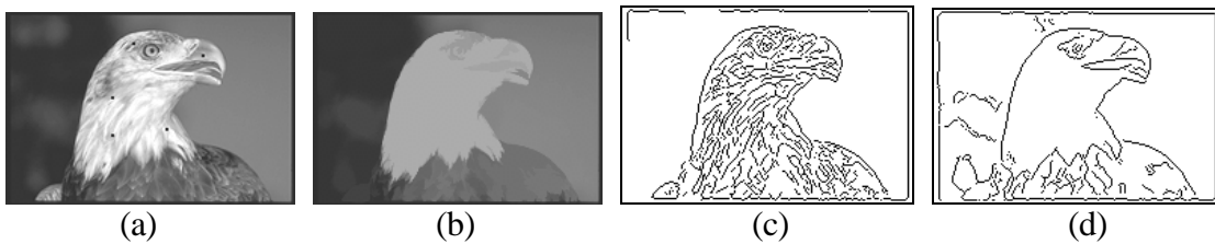
Figure 5 (a) A bird image. The user has mouse-clicked inside the head and neck of the bird (5 black dots). (b) After inclusion filtering the image with the markers (5 black dots). (c) edges of (a). (d) edges of (b).
