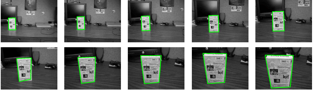
Figure 8 Successful tracking within a real closure sequence with the projection object model.
