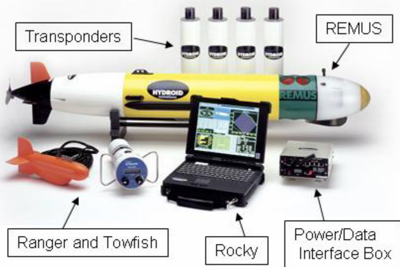
Figure 2. REMUS and Equipment, after Hydroid, Inc. (2003)
