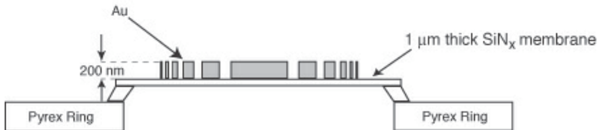
Figure 3- 22. Schematic of an X-ray mask.
