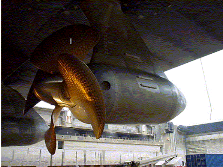
Figure 5. ALSTOM 20MW Azimuth Pod (Mermaid™) [From Ref. 5.]
