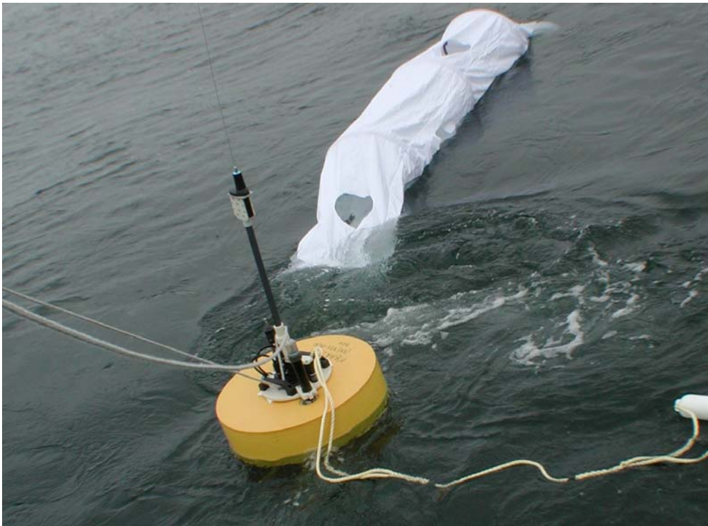
Figure 6. Drifter with Its Drogue Shortly After Deployment.
