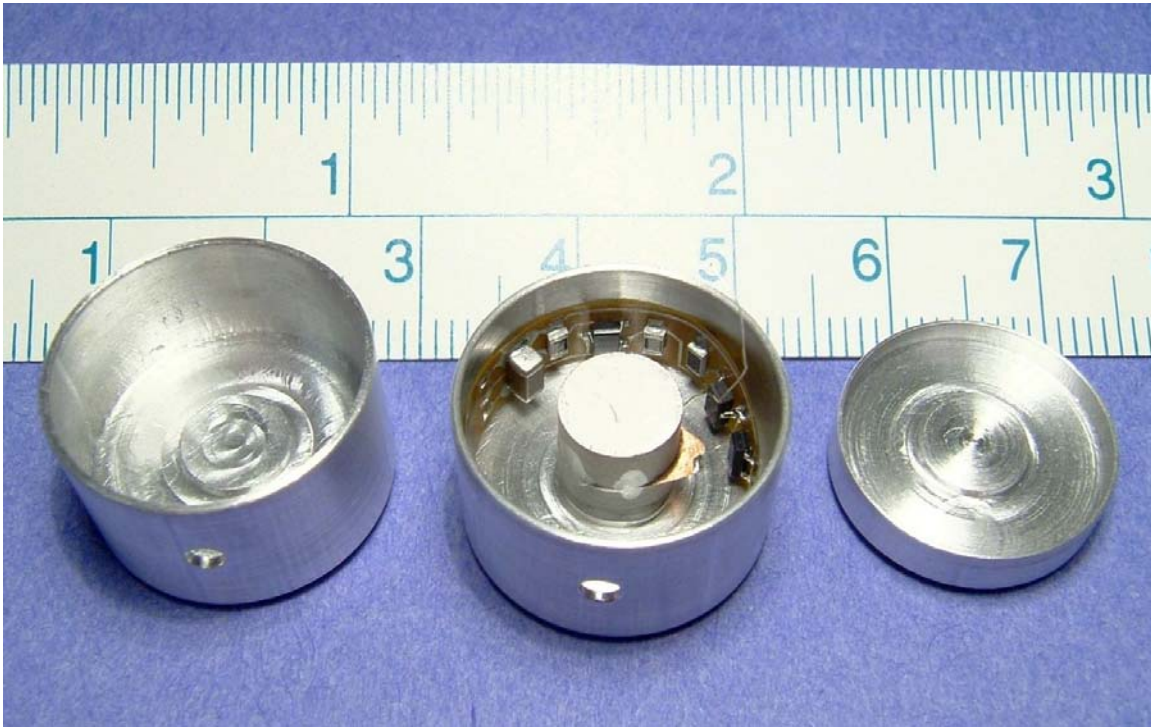
Figure 12. Aluminum parts of MiniCan-7 with PZT stack and the flexible preamplifier already mounted inside the base.
