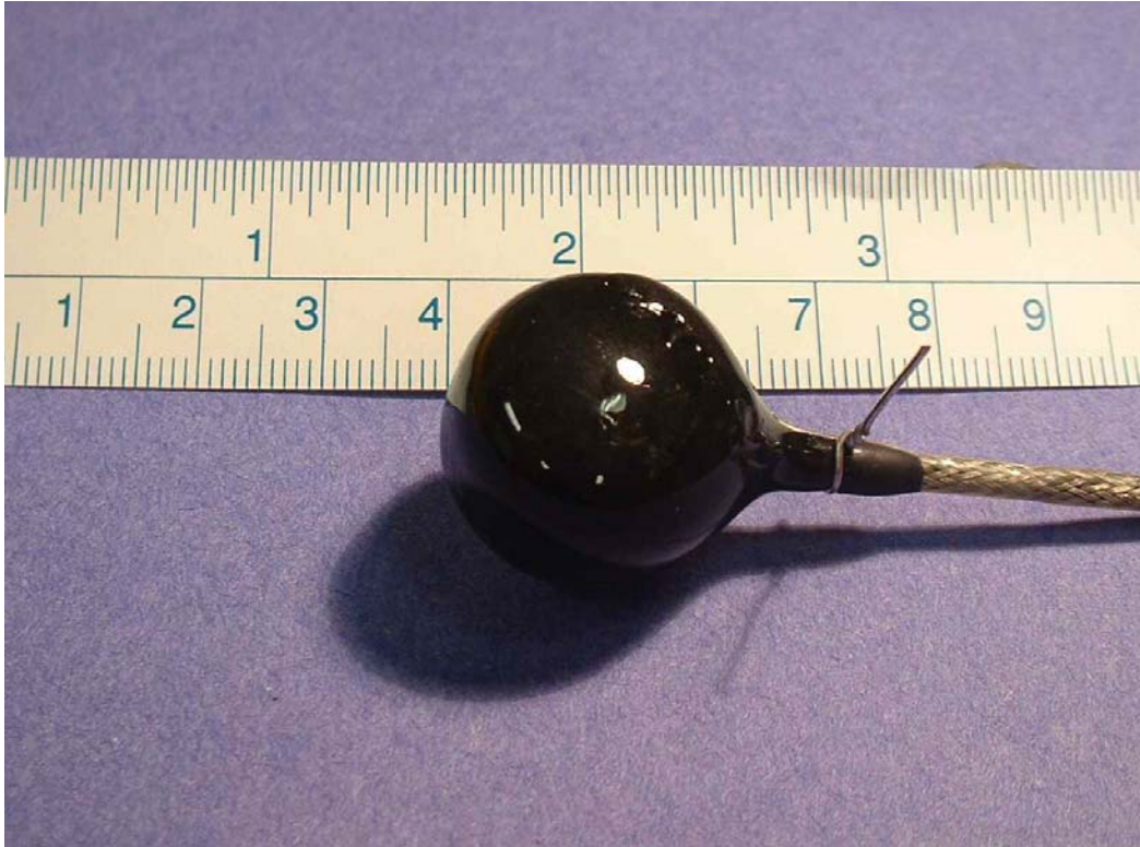
Figure 13. Assembled MiniCan-7 Hydrophone ready to start underwater measurements.
