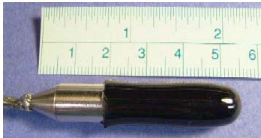
Figure 9. Hydrophone Partially Covered with Polyurethane
