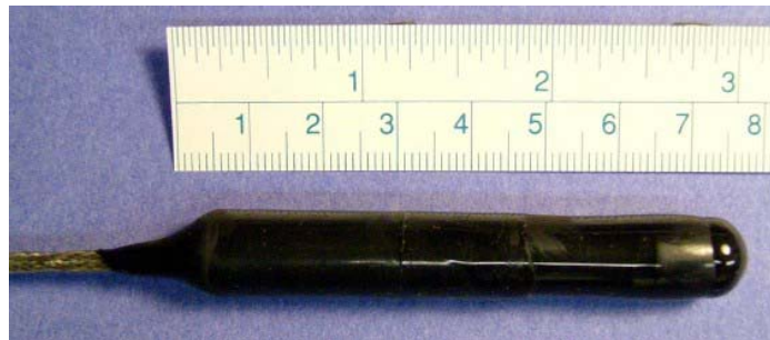
Figure 10. Hydrophone Totally Covered with Polyurethane
