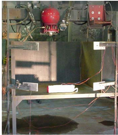
Figure 1: Suppression System and Table with M3 Propellant
