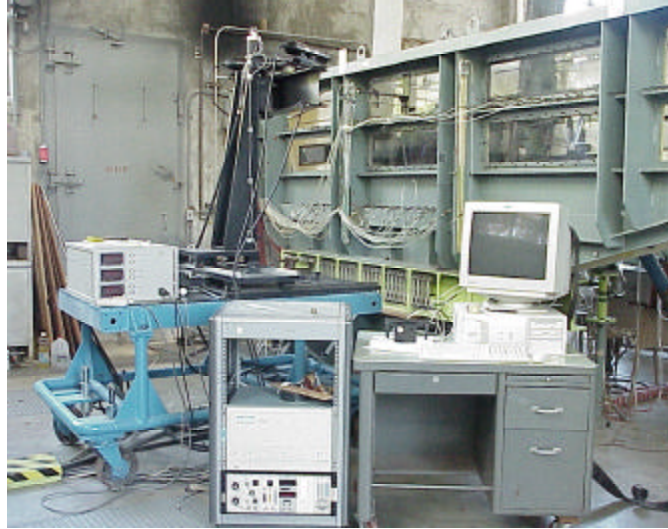
Figure 7. Optical Probes, Traverse Table and Data Acquisition System
