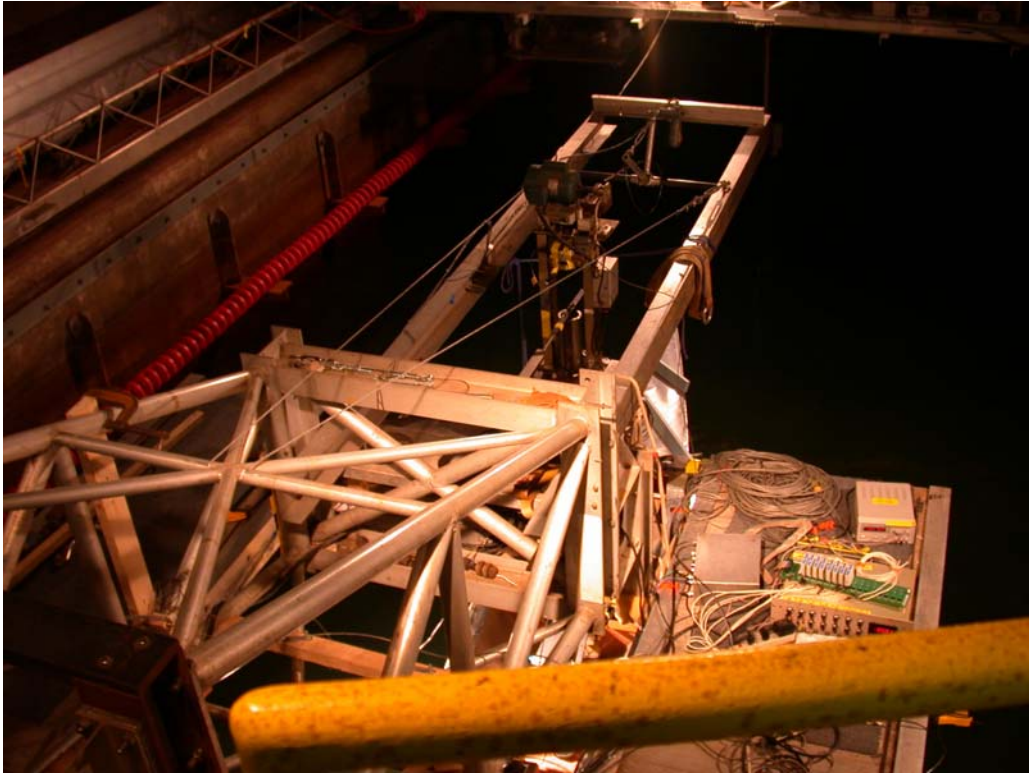
Figure 24: Carriage 3—David Taylor Model Basin Cantilever Model Jig
