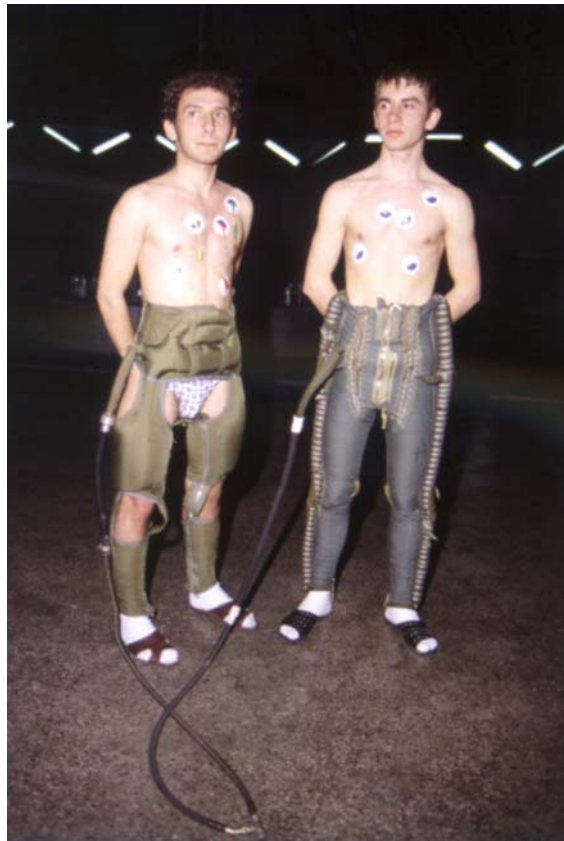
Fig. 1. Anti-G suits used in Polish aviation – left is PPK – right is WUK
