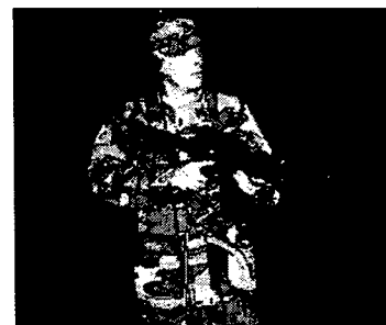
Soldiers in the virtual environment carry a modified M4 rifle that also holds the controls for other weaponry and devices. The Soldier is wired with sensors that communicate his position and posture to the simulation system, which then portrays the Soldier realistically in the virtual environment.
