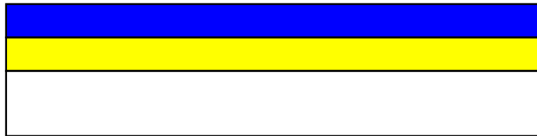
1. Oxide and poly deposition
