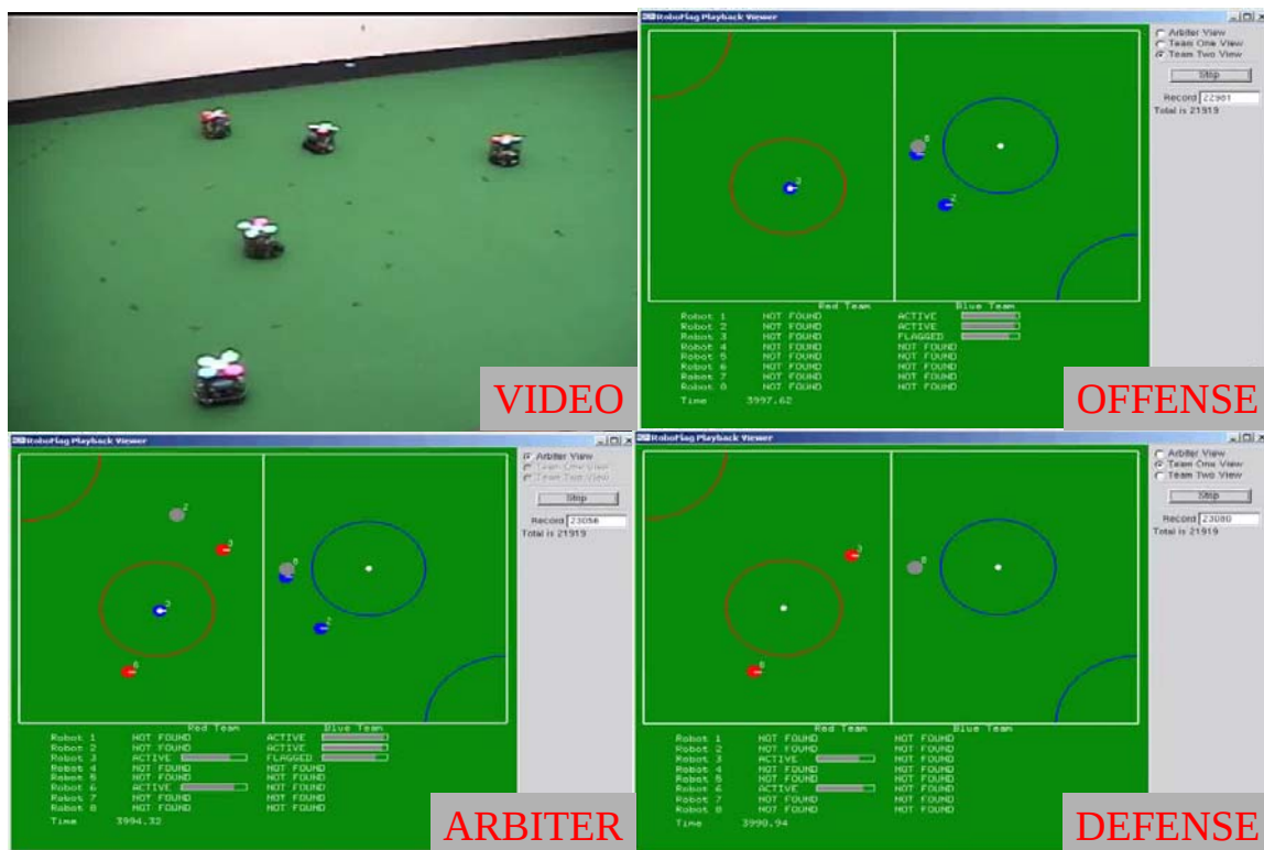
Figure 17: Four views of a typical RoboFlag game. Upper left: a video of the hardware running. Lower left: an arbiter view of the game, which represents all aspects of the system. Upper Right: An offense (blue) view of the game; note that blue can only see its own team now, based on its smaller sensor radii. Lower Right: An defense (red) view of the game; note that red can only see its own team now, based on its smaller sensor radii.
