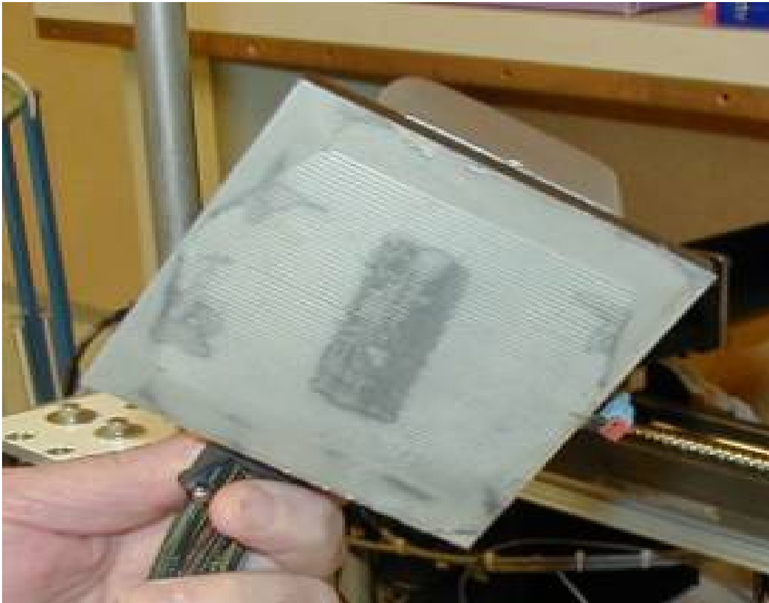
Figure 13. Scanning surface of 64-element array head. (Note: The ribbon like traces, which launch the unidirectional current sheet into the sample. The angle between the string orientation and the scan direction can also be seen through the Mylar excitation unit, showing its thinness. The return traces are located at the top and bottom of the unit, and are bunched more closely together than the excitation traces.)
