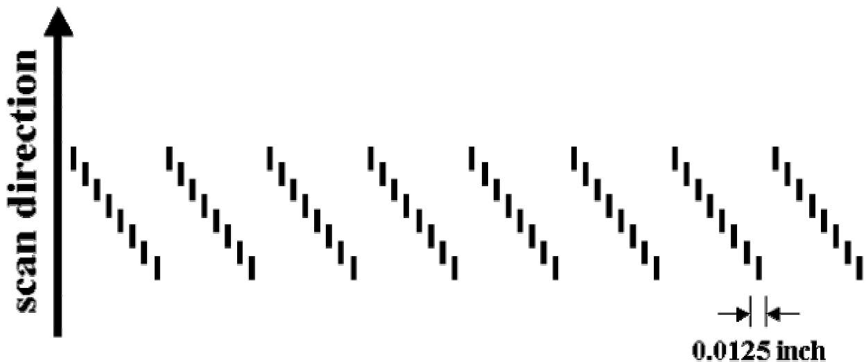
Figure 7. Configuration of 64-element array per the spacing conditions: The inter-sensor spacing is 0.0125 inch, normal to the scan direction.
