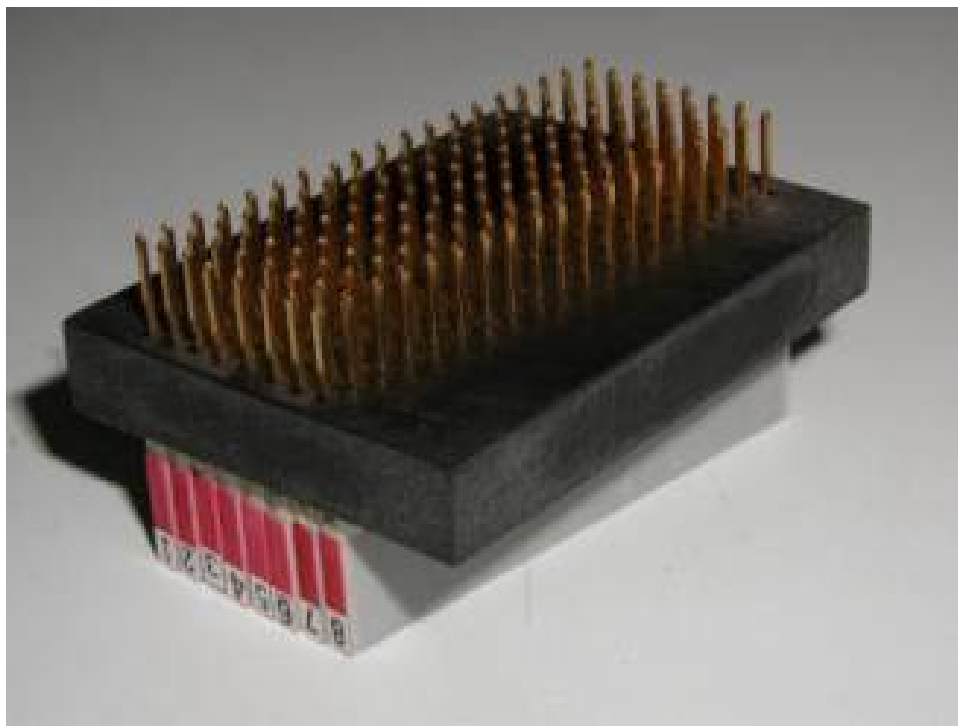
Figure 11. 64-element array, shown without its metal shield, with eight strings of sensors and 8x19 pins protruding through the Delryn mounting mandrel.
