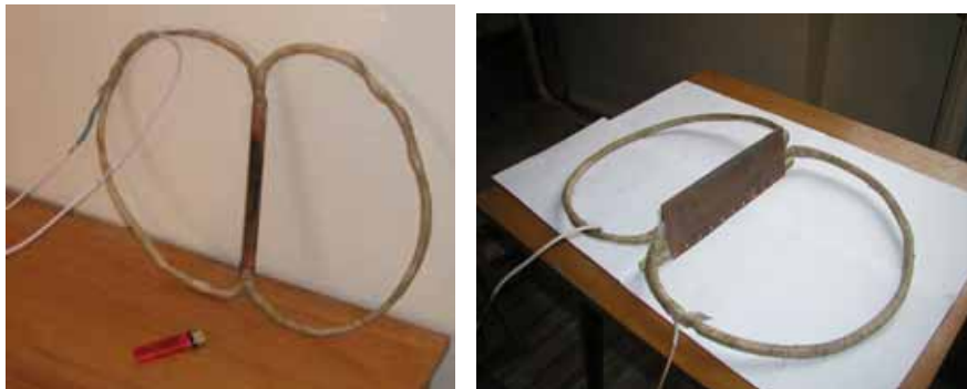
Figure 2 Circular Cylinder (left) and Single Angle Wedge Models used in MHD External Flow Control Experimental and Theoretical Studies (IVTAN-TsAGI-CIAM team)
