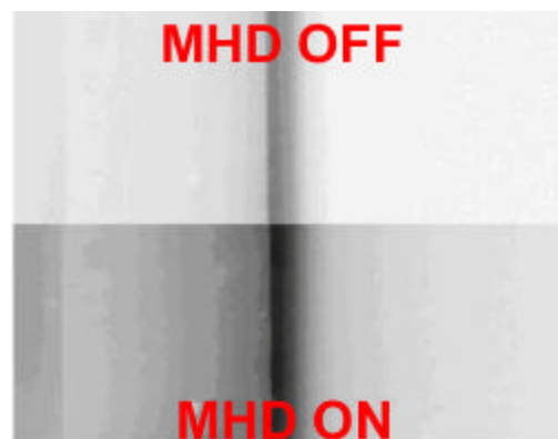
Fig.19. Imaging of the flow around cylinder with and without MHD interaction as recorded with Pulnix digital camera. The flow direction is from the right to the left.
