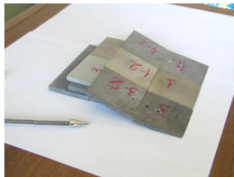
Figure 36. The 'double angle' wedge model at the assemblage.
