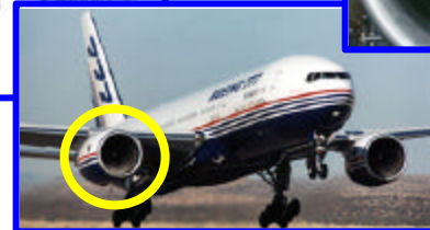
DRA has replaced gr/epoxy fan exit guide vanes in PW 4XXX engines
