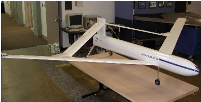
Figure 2: The Joined Wing Technology Demonstrator as Delivered Under Contract with AeroComposites, Inc.
