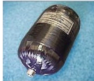
9700 psi TVC tank for Delta Rocket
