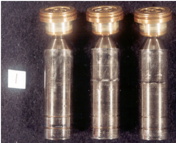
Pistons 1-3 at 1515 Hours Fresh Fluid
