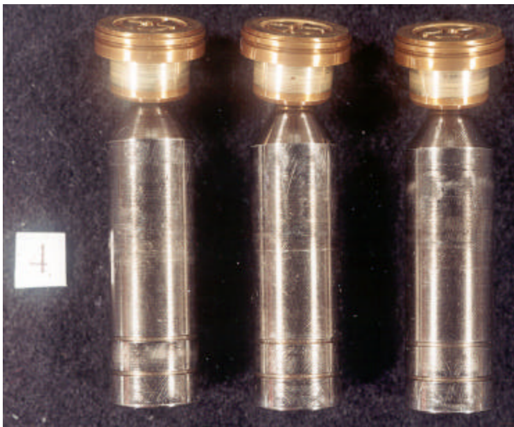
Pistons 4-6 at 1515 Hours Fresh Fluid
