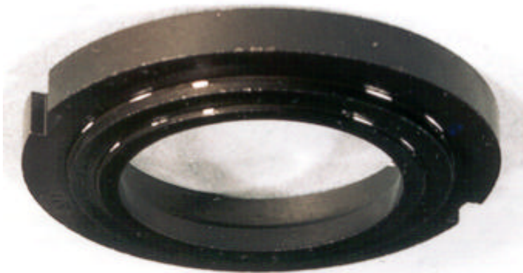
Shaft Seal at Pretest Purified Fluid
