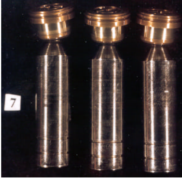
Pistons 7-9 at Pretest Fresh Fluid
