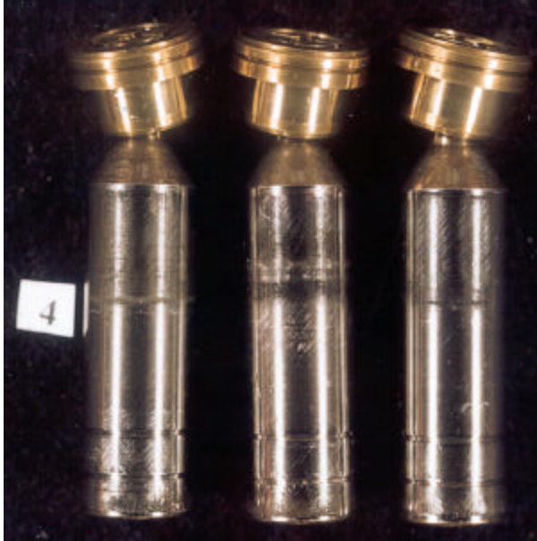
Pistons 4-6 at Pretest Purified Fluid
