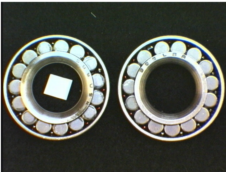
Pintle Bearings at 1500 Hours Purified Fluid [white square denotes case drain outlet side]
