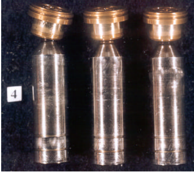
Pistons 4-6 at Pretest Fresh Fluid
