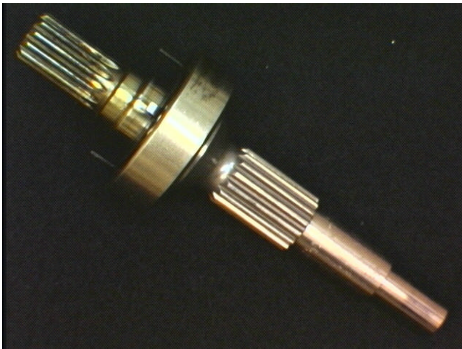
Shaft at 1500 Hours Purified Fluid
