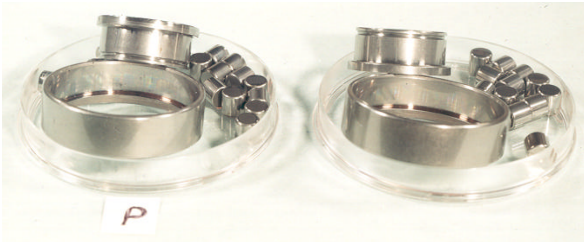
Yoke Pintle Bearings at 1515 Hours Fresh Fluid [white square denotes case drain outlet side]
