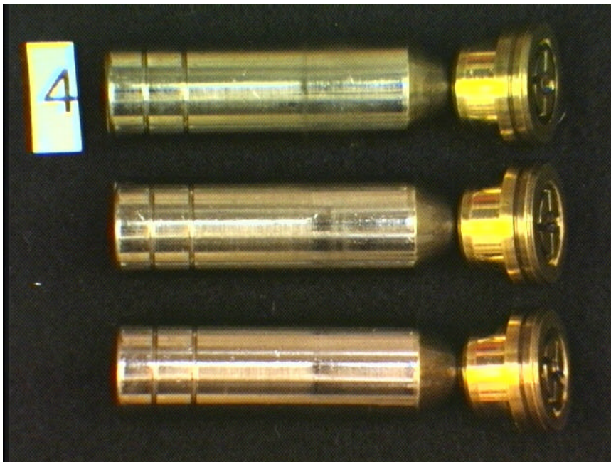
Pistons 4-6 at 1500 Hours Purified Fluid
