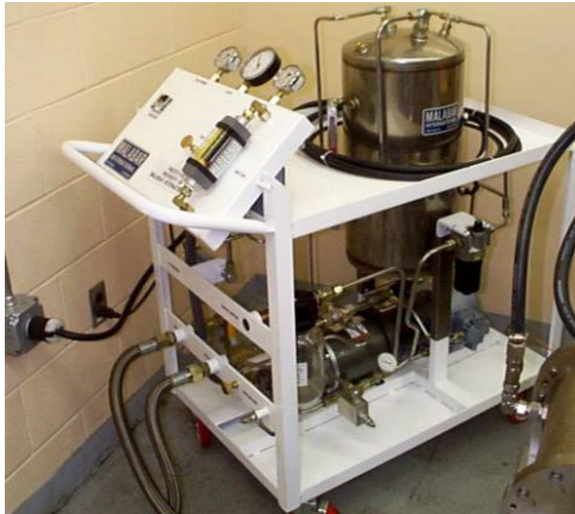
Fig. 2 Malabar Purifier Mounted to a Portable Cart
