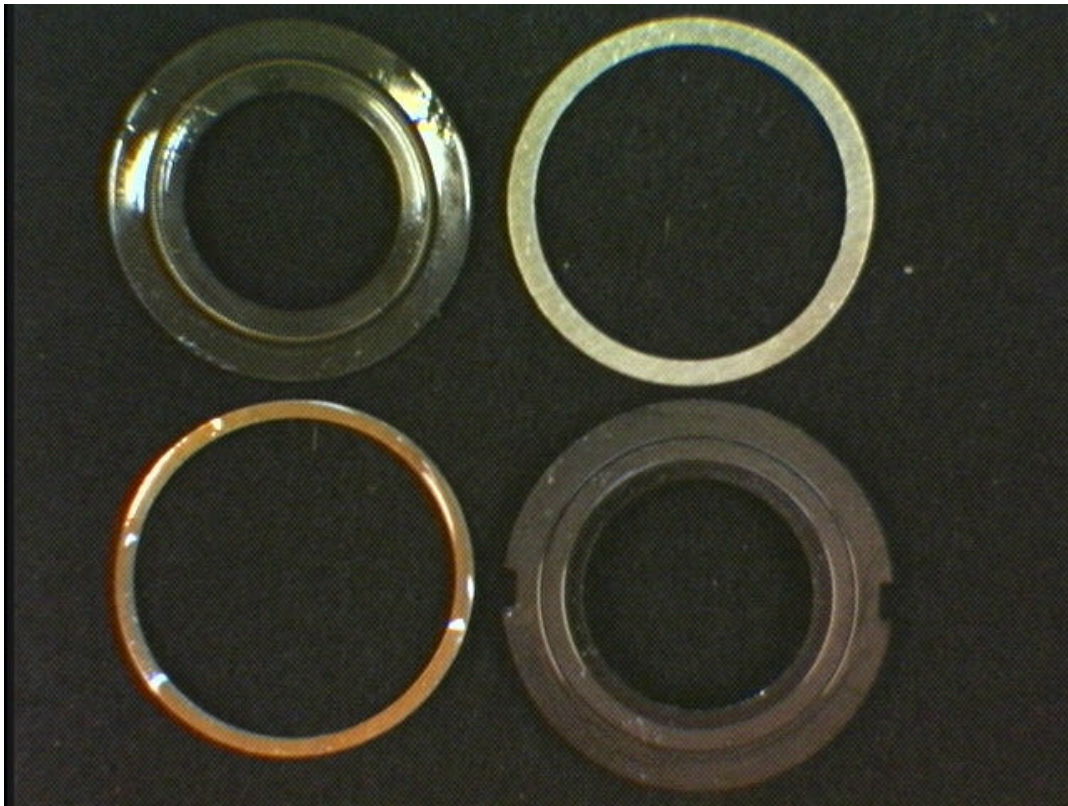
Shaft Seal at 1500 Hours Purified Fluid
