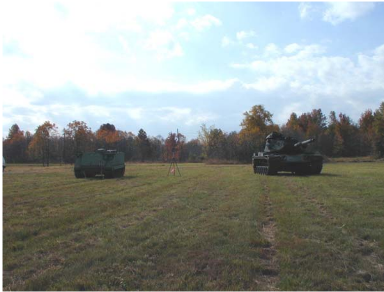
Figure 2: Run 7, both tanks at the same down-range distance measured from center of the radar to the approximate target centroids.
