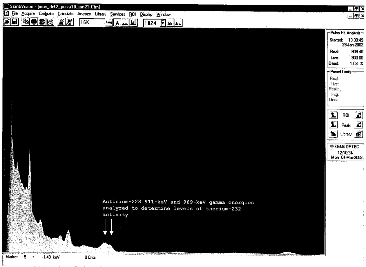
Figure 7. NaI gamma detector spectrum of 50-pCi/g calibration disk. The arrows denote the gamma energy lines of actinium-228 used to determine levels of thorium-232 activity
