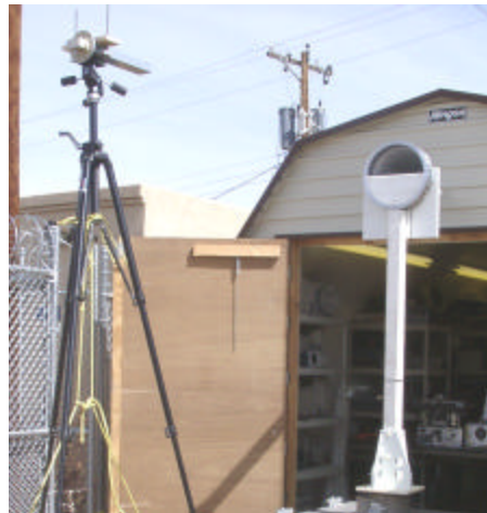
Figure 10. Pattern measurement configuration.
