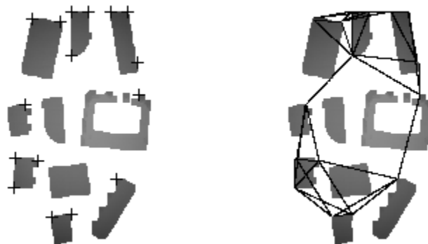
Figure 4. Landmarks and scene graph for range data acquired with a structured light sensor.
