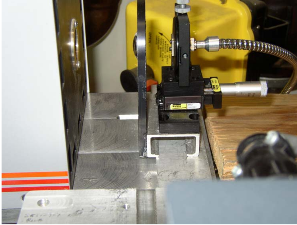
Figure 3: Side View of Blackbody Connection Assembly (Point 1)
