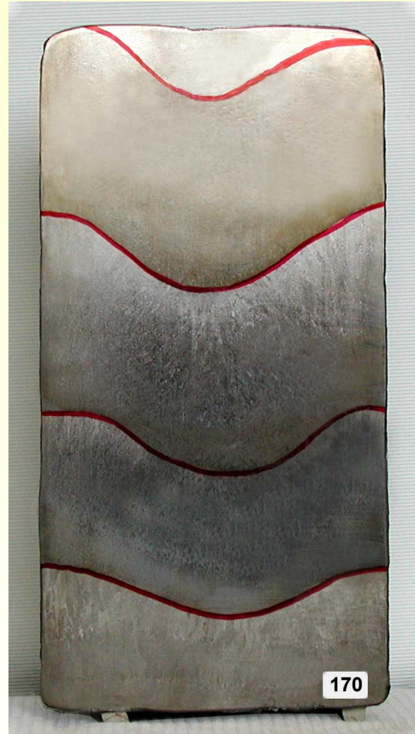
Shape of metal pool during melting in transversal magnetic field
