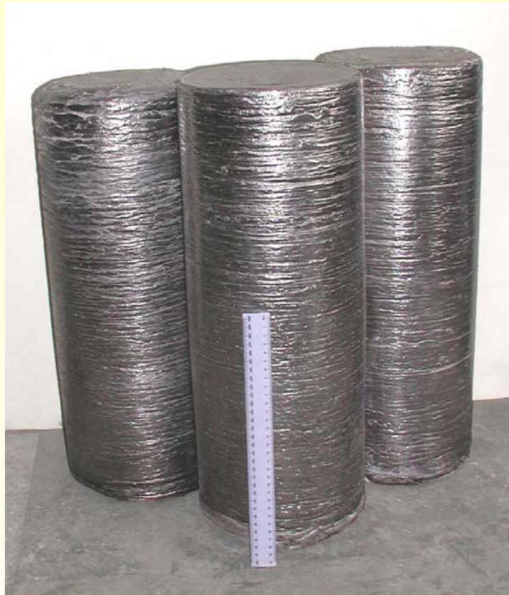
Ingots of alloy Ti-10-2-3 with a diameter of 220 mm by MEM technology
