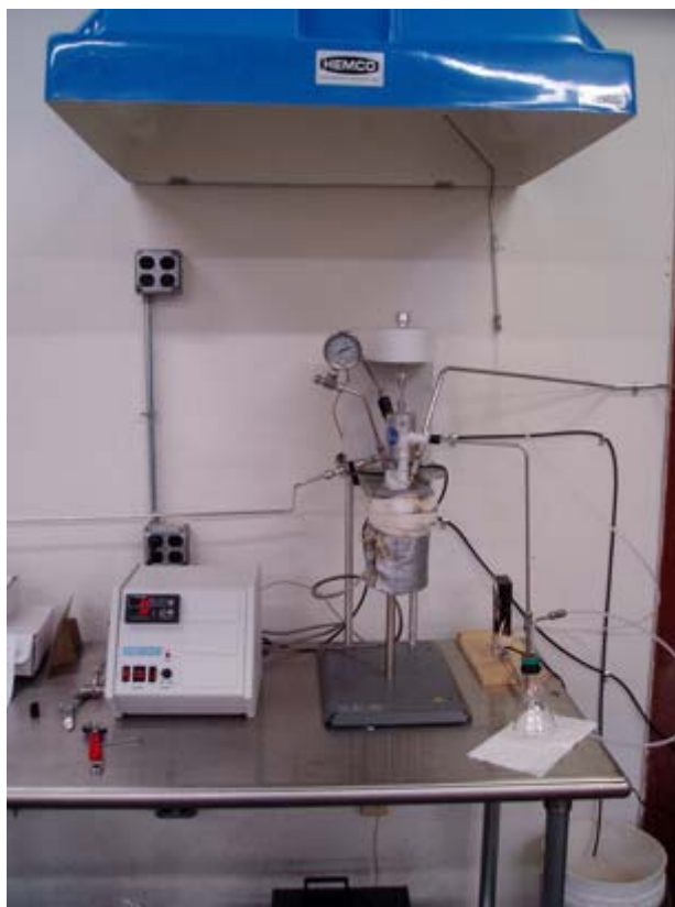
Figure 5. Parr reactor apparatus. The liquid product trap and gas flow meter are to the right of the reactor stand.
