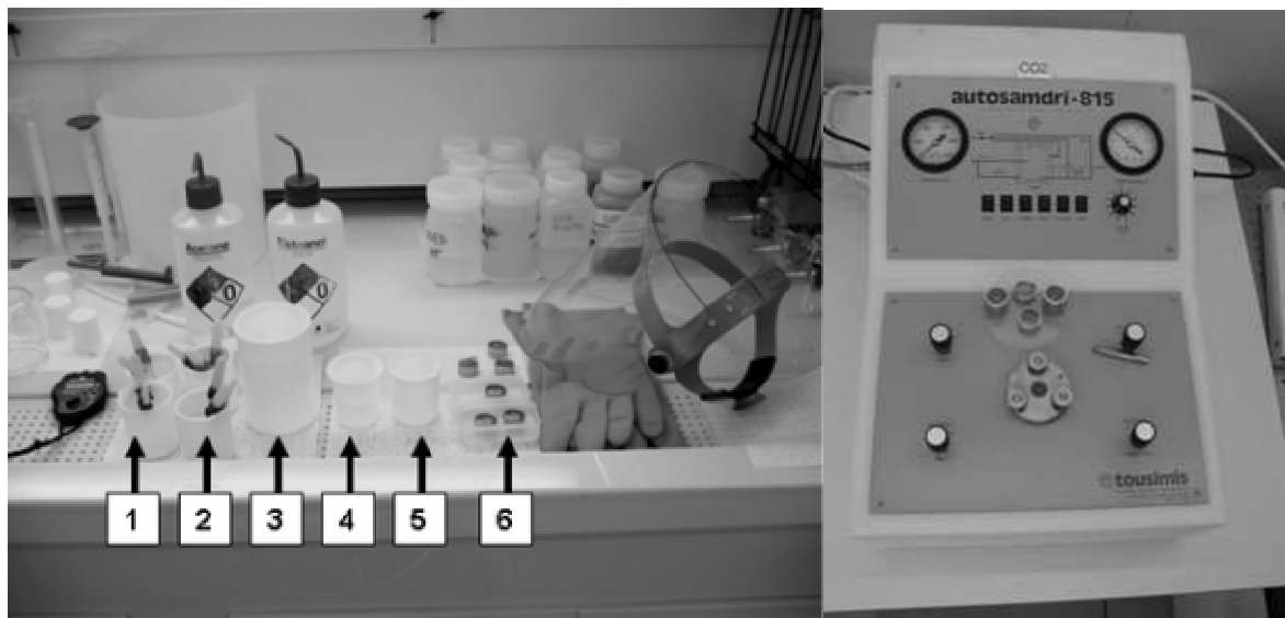
Figure 6.2: Photographs of the PolyMUMPs HF release setup, with (a) being the chemicals and safety equipment and (b) being the CO 2 critical point dryer.
