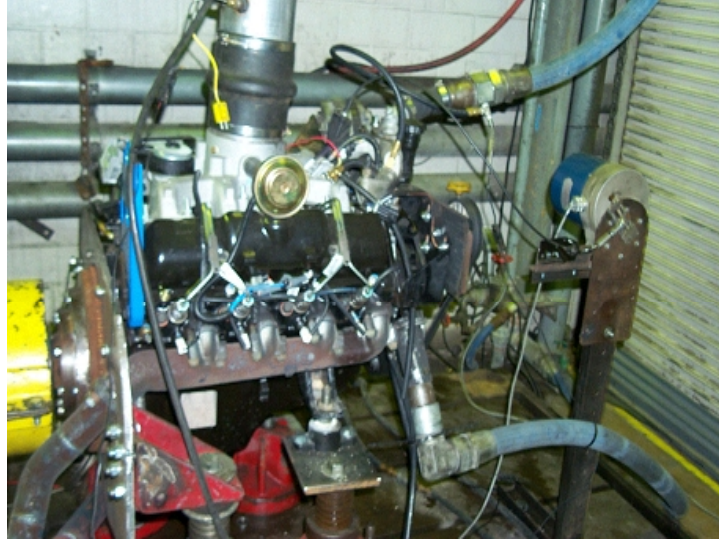
Figure 1. Installed 6.5L Heavy-Duty Diesel Engine
