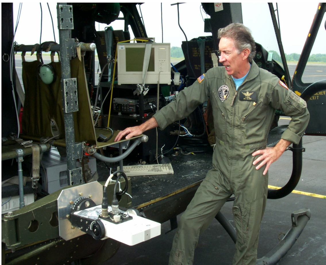
Figure 2. The downward-looking Weibel radar head configuration.
