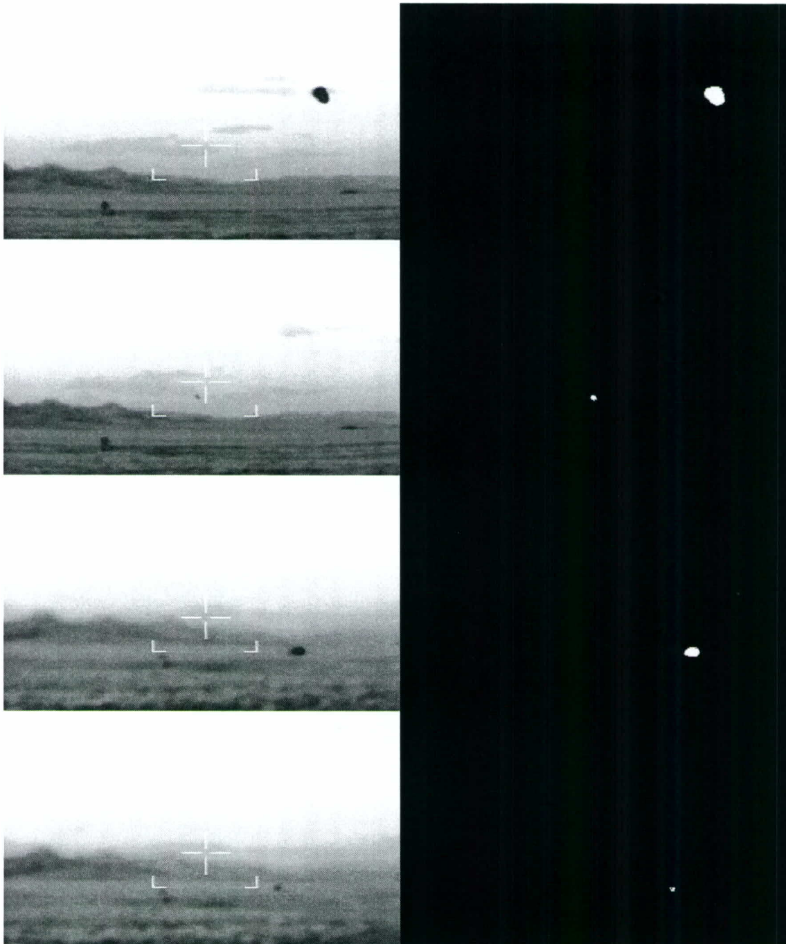
Figure 7. Images from the 10 th Frame After Detonation. Top to Bottom: HE Airburst, CB Airburst, HE Point Detonation, and CB Point Detonation
