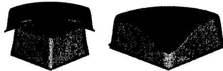
Figure 16: Optimal preform and final forged product for the closed die forging problem.
