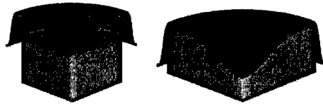
Figure 15: Initial preform and final forged product for the closed die forging problem.
