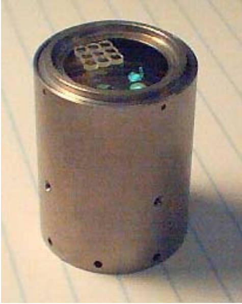
Figure 3-3. Lens barrel containing multi-scale optical elements for global multi-chip interconnections. Macro-optical elements are the size of the barrel, whereas an array of mini-optical elements is mounted to an optical flat in the barrel
