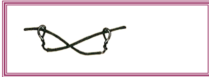
Figure E-7: Pull-Loop Switch (Source: TM 31-210)
