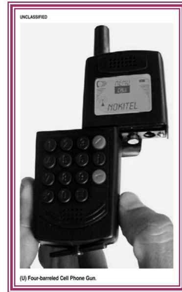
Figure E-21: Four-barreled Cell Phone Gun (Source: File Photo)
