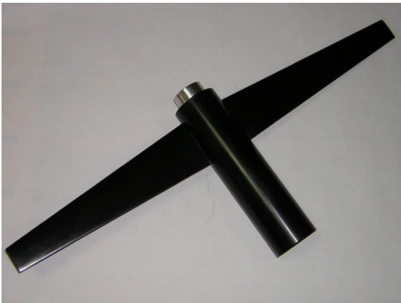
Figure 8.7 – Main part of the winged model (“trapezoidal wing-fuselage” variant)
