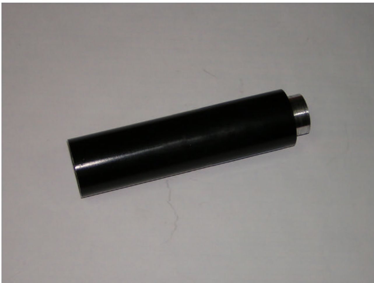
Figure 8.6 – Main part of the model fuselage (“clean fuselage” variant)
