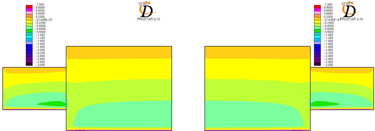
Figure 7.17 – Pressure coefficient distribution for lower and upper surface of the telescope wing, \alpha = 0^\circ
