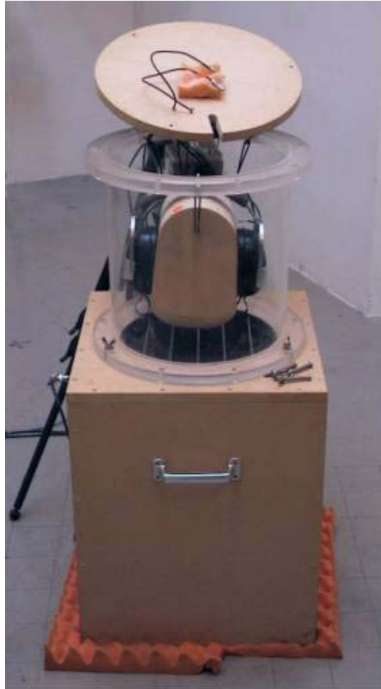
Figure 6: Dummy Head with “Flat-Plate” Microphone in a Volume Suitable for Relatively High Noise Levels (130 dBA).
