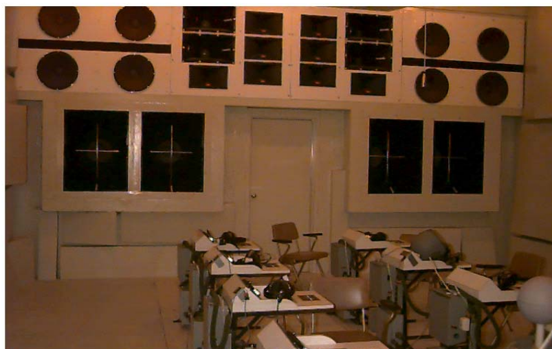
Figure 7: High Noise Listening Room at AFRL/HECB. The room is used for MRT listening tests.
