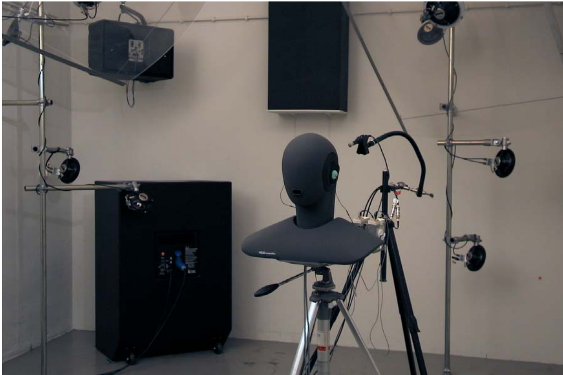
Figure 3: Artificial head placed in a high noise room, designed for generation of a diffuse sound field (max. 120 dBA). Two of the five high power loudspeakers (back view) are visible at the left. In the center of the wall a sound absorption module is placed. The small loudspeakers are not used (these are available for hearing threshold experiments).
