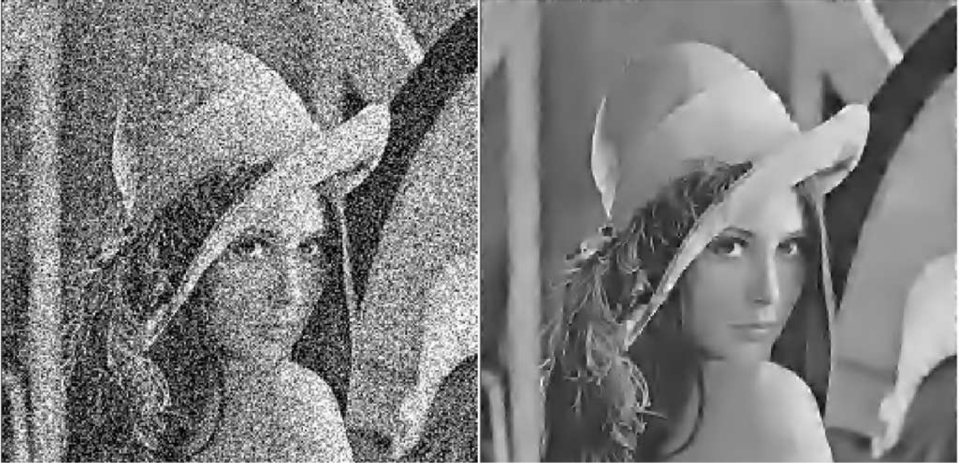
Fig. 5. Optimal denoising method applied to noisy "Lenna" image. Left: Corrupted image \tilde{f}(x, y) , \sigma_n = 50 , PSNR = 14.16 dB. Right: Optimally denoised image f^{opt}(x, y) , PSNR = 27.72 dB.
