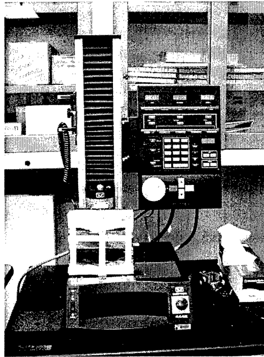
FIGURE 2.13: Picture of Instron machine and test setup.
