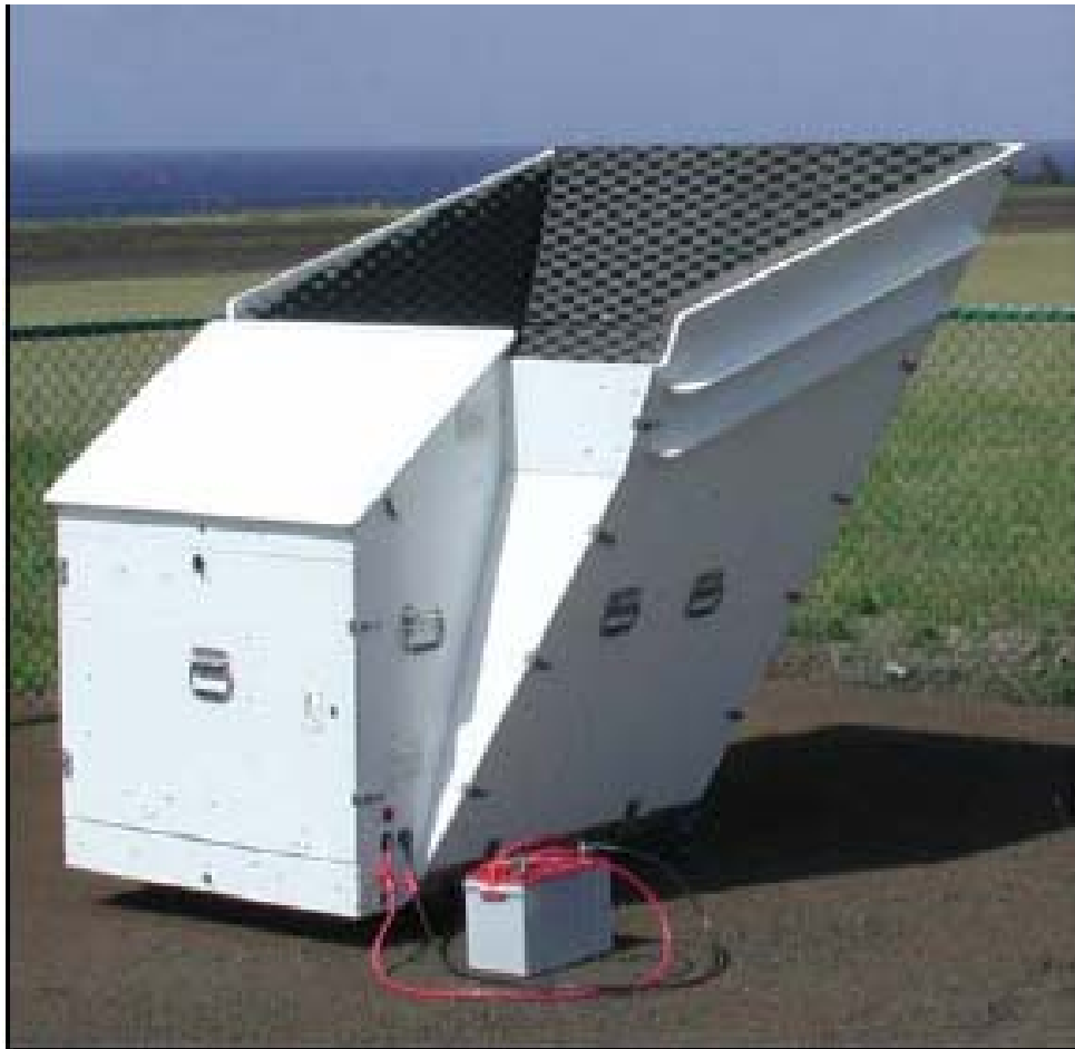
Figure 1. Model VT-1 phased-array doppler sodar system.
