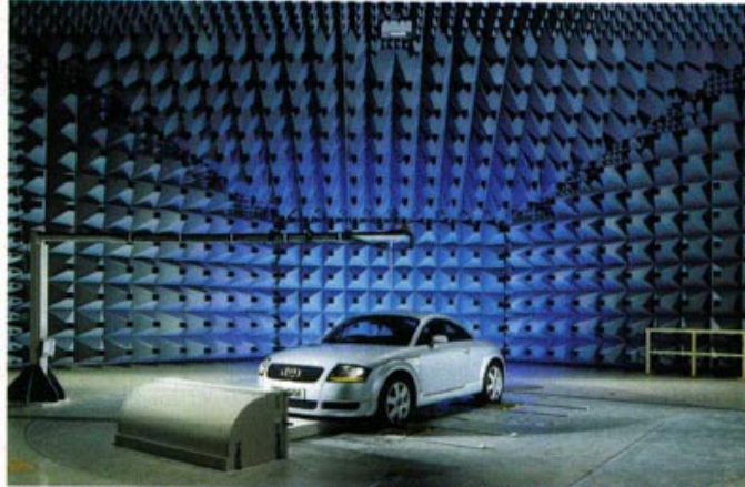
Figure 3. Automotive electromagnetic compatibility testing (From Ref. [1]).
