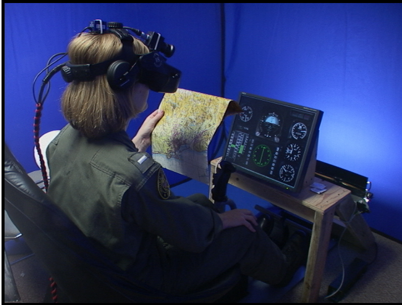
Figure 6. Student in Mock Cockpit with Blue Screen Matting.
