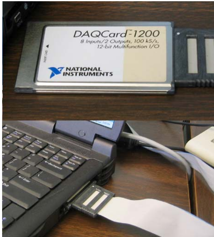
Figure V-5. The data acquisition card (top) inserted into the laptop's PCMCIA port (bottom).
