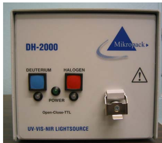
Figure IV-4. Ocean Optics DH-2000-CAL calibration lamp. The metal cover toward the lower right is covering the fiber cable insertion hole.
