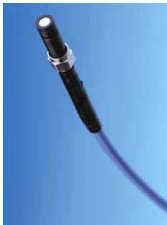
Figure IV-3. Fiber optic cable with cosine corrector attached at its tip (the black/white item at the end of the cable). The white element is the Teflon diffusing material (From [23]).
