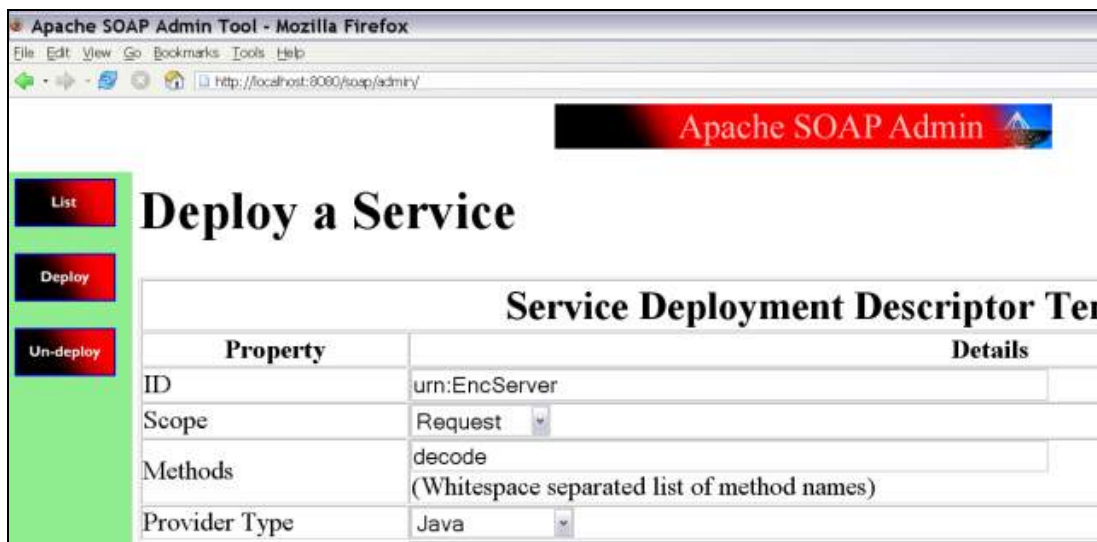
Figure 23. This screenshot shows the service deployment descriptor ID and methods list configuration form. These parameters are used to create the service deployment descriptor file used by SOAP.
