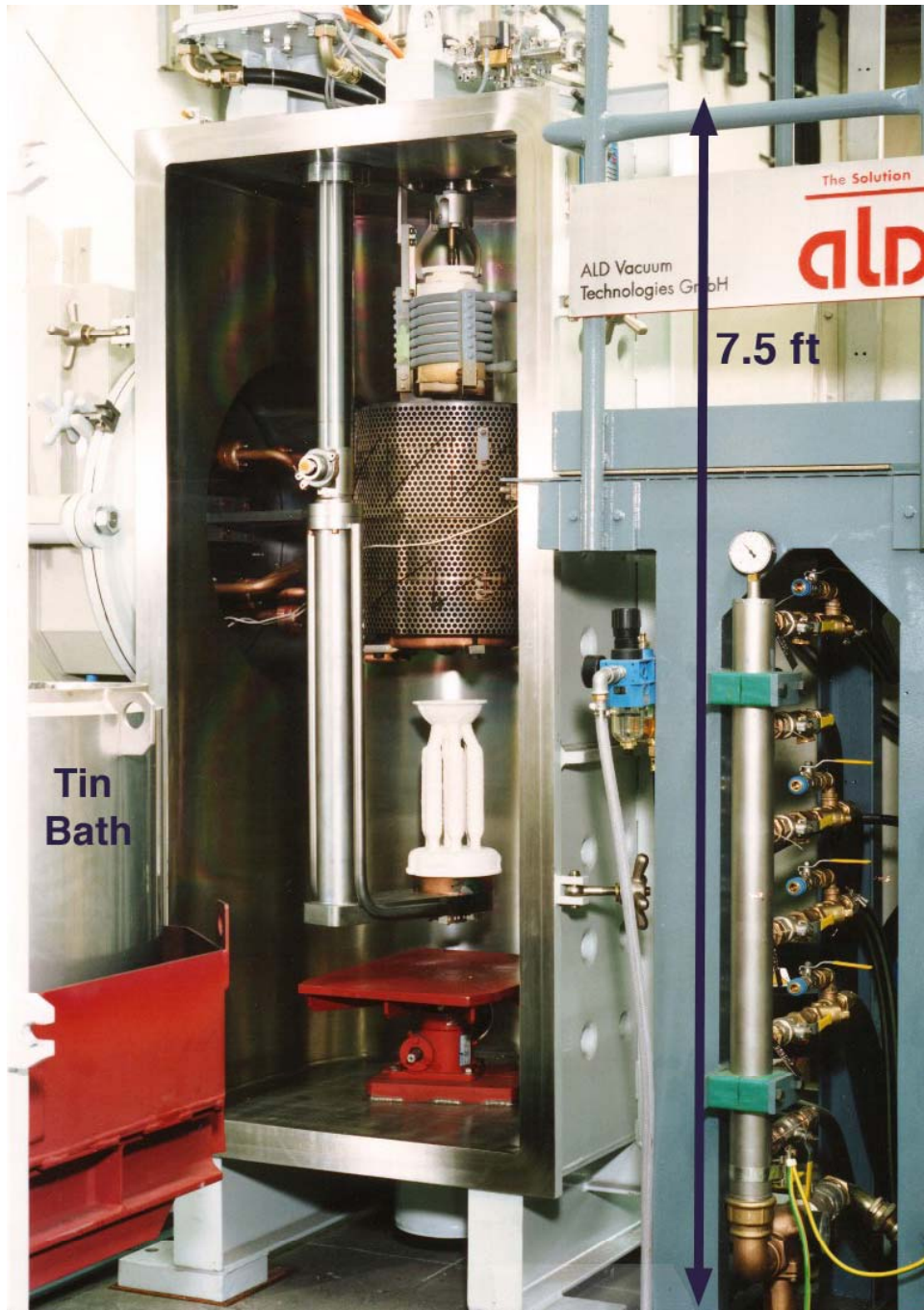
Figure 1 – Chamber of the Bridgman/LMC-Sn system at the University of Michigan. The tin bath is supported by the outer door (to the left). Crucibles are top loaded into the 50kW induction coiled, melted and bottom poured into the the preheated investment mold.
