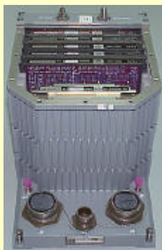
MPCA* (Modular Central Processing Assembly)
