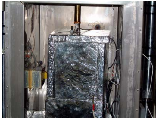
Figure 17. Insulative Chamber around Test Specimen
