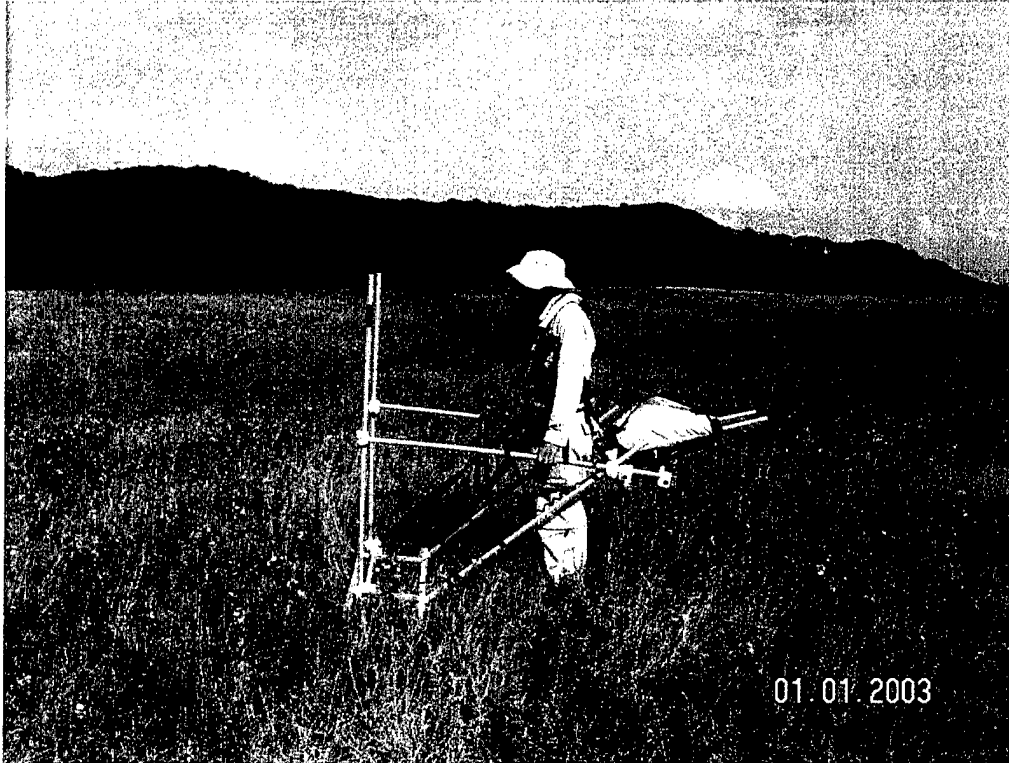
Figure 1. Demonstrator's system, TM-5 EMU (dual sensor).
