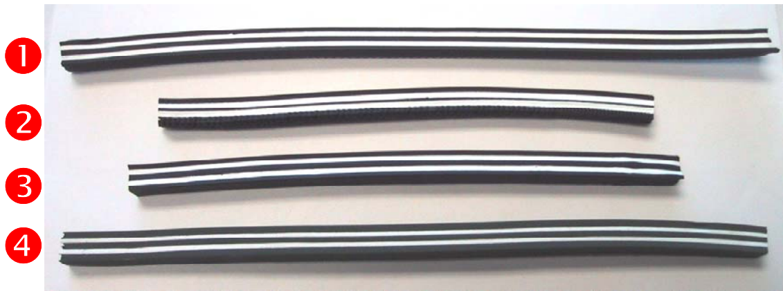
Figure C12. Extruded hybrid honeycombs of YSZ and different interconnect: (1) Fe39Ni8Cr, (2) Fe15Cr, (3) Fe10Cr15Ni, and (4) Ni18Cr10Co5Mo.
