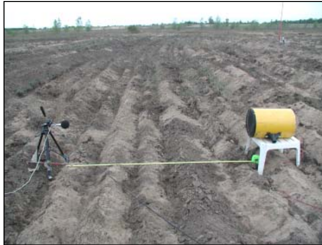
Figure 20. Impedance measurements of the plowed-field surface.
