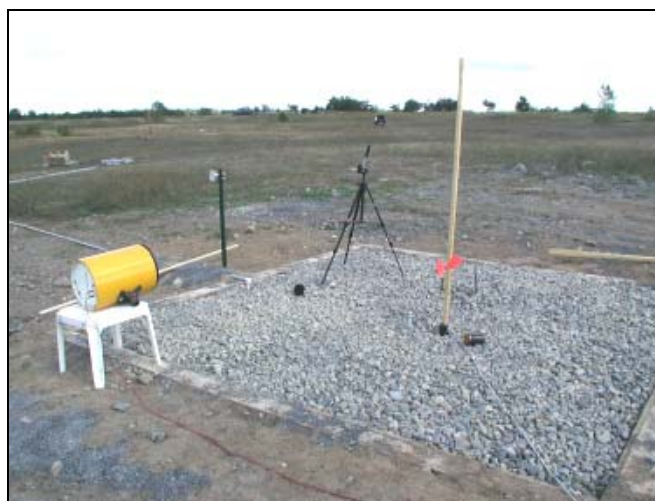
Figure 19. Impedance measurements of the Pit 1 surface.
